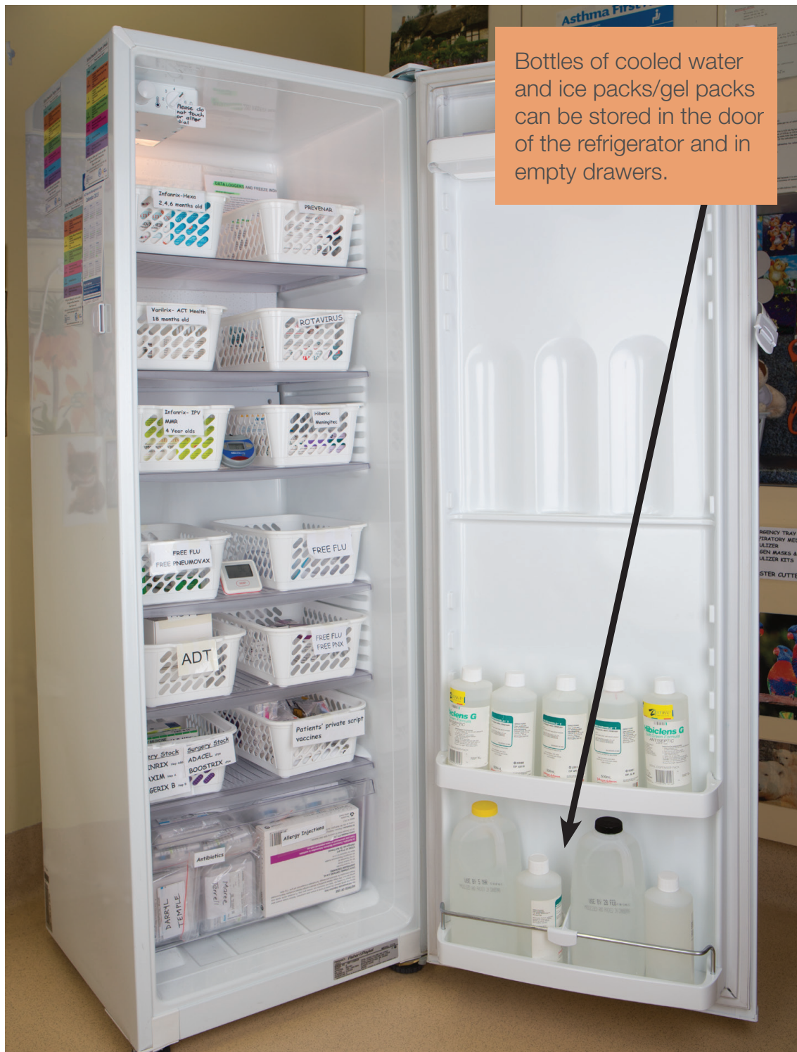
Figure 6: Modification of a domestic refrigerator
